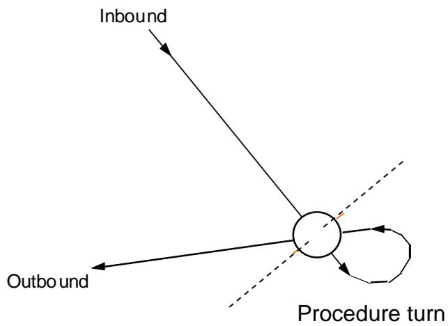
A procedure turn is mandatory at a turning point (TP) in case of a change of track of more than 90 degrees
